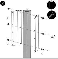
Assemble the post clamping brackets together using 3 x M8 bolts and nuts using 5mm Allen key.
