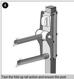
Test the fold up rail action and ensure the post and frame is stable and does not move. Further height adjustment maybe required by adjusting the bracket.
