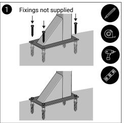
Pre-assemble and check all parts are present. Determine the positioning of the post and fold up rail. Mark the floor position using the pre-drilled holes in the floor plate. Drill suitable sized holes and insert the floor anchors. Mount the post to the floor using suitable floor mounting screws or bolts.
